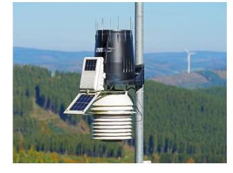
It will be cable to measure the temperature, the relative air humidity but most interesting: the PM10 and PM2,5.
